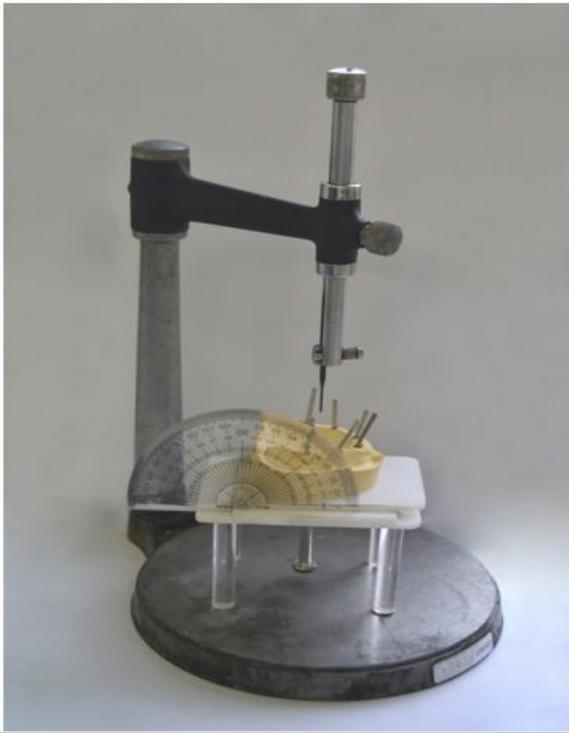
**Figure 4:** Full measuring apparatus setup. Analyzing rod attached to tool holder.
