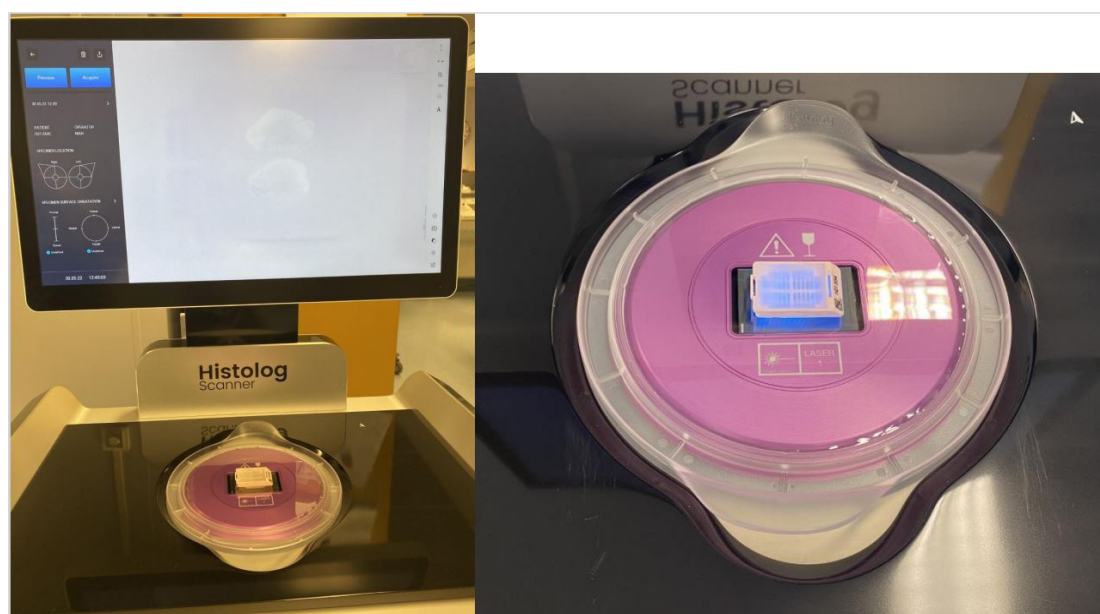
Figure 1: Overview of the Histolog® Scanner device with a broached FFPE block on the scanning surface.
